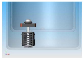
Figure 16.4b. CAD Drawing of Open Valve
